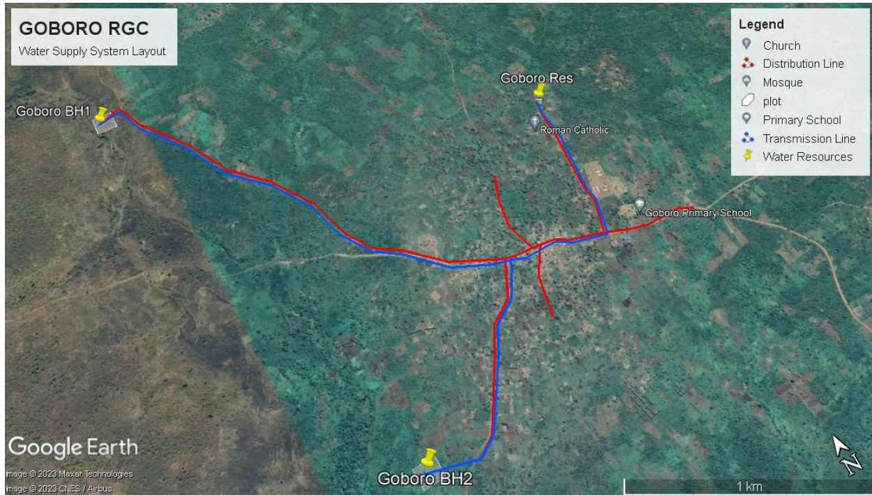
Figure: 3-2: Goboro RGC Water Supply System Schematic Diagram
