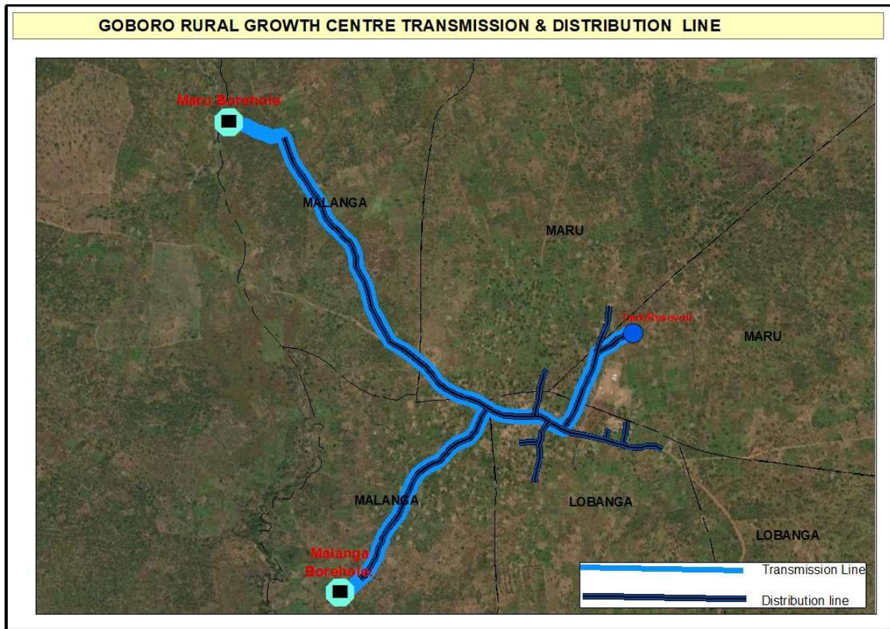
Figure: 1-6: Water transmission and distribution route
