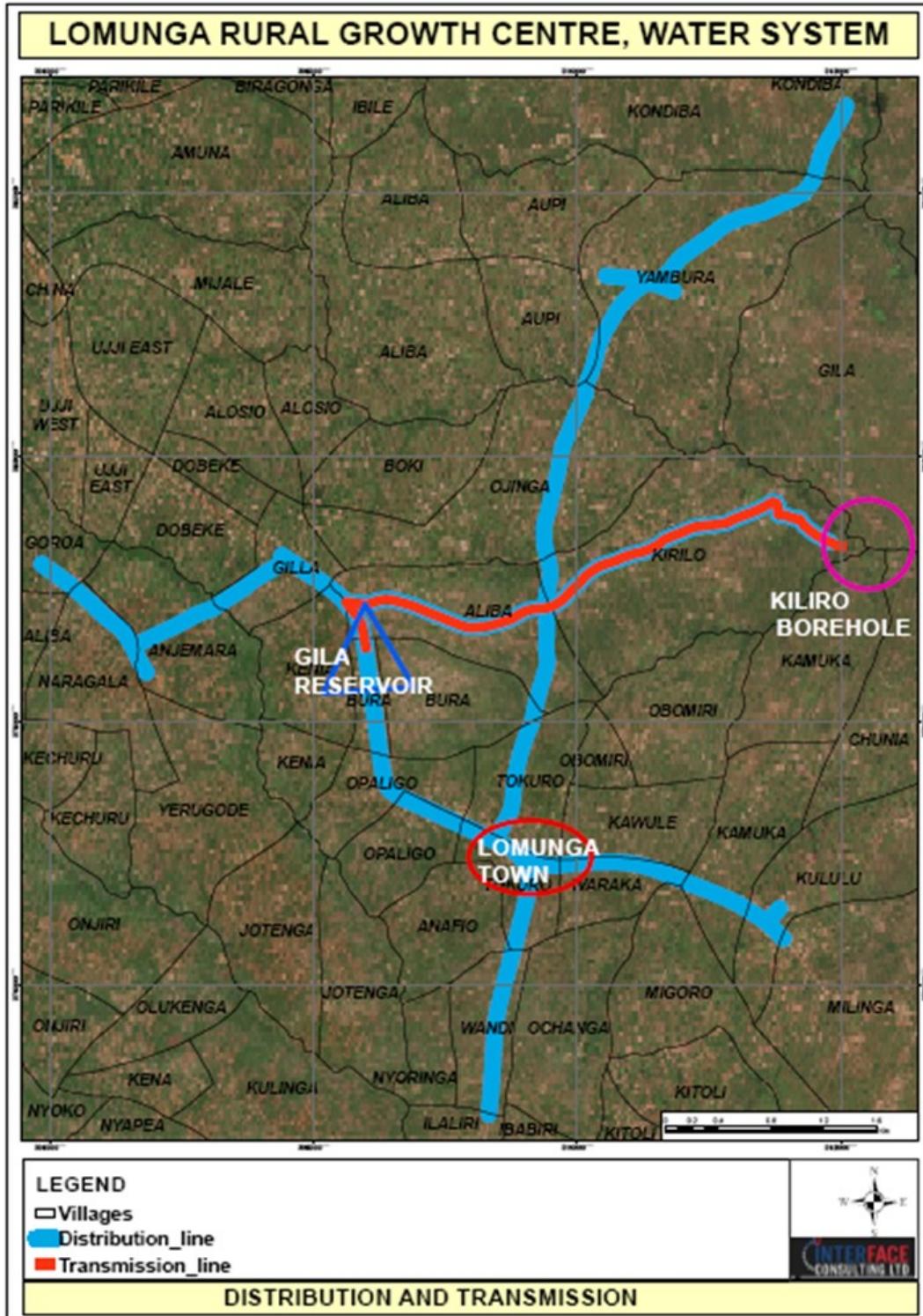
Figure 1-1: Water Transmission and Distribution Network
