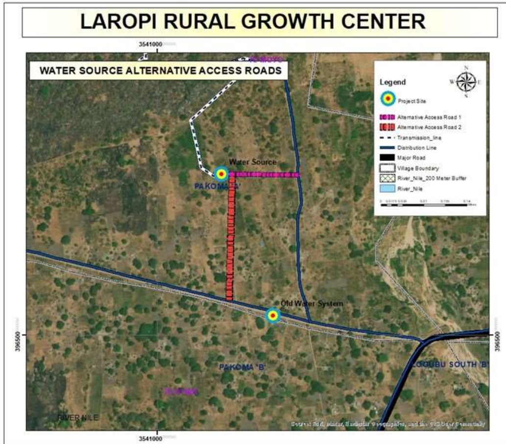
Figure 5-1: Alternative Access to Water Source.
