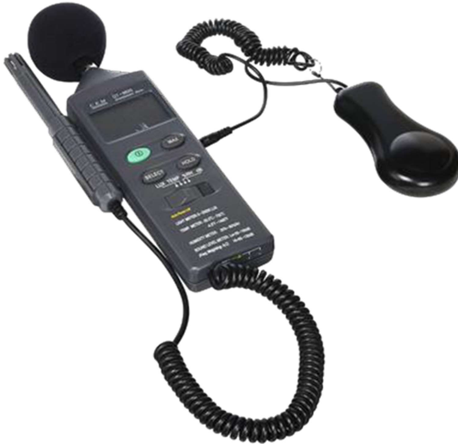
Figure 2-2: Handheld Sound Level Meter, Light Meter, Humidity Meter, and Temperature Meter (CEM DT-8820 Environment Meter)
