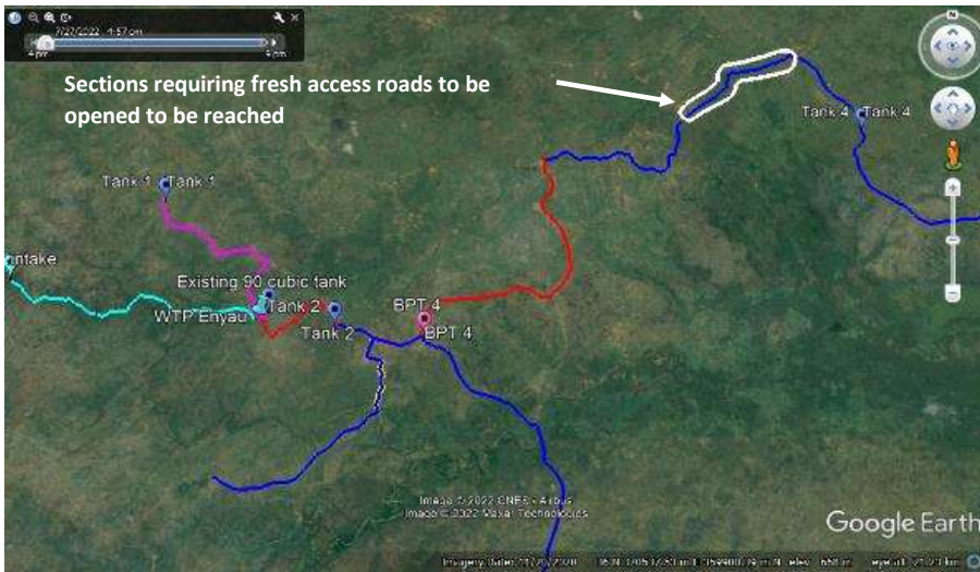
Figure 2.4: Enyau WSS infrastructure routes with poor road infrastructure (fresh access road to be opened)
