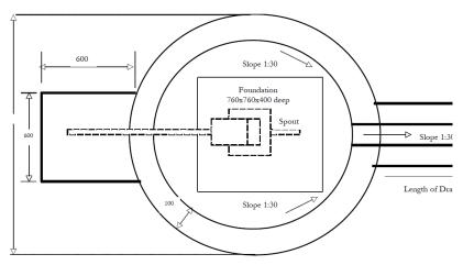
Figure 5: A U3M pump on a sealed borehole with concrete apron
