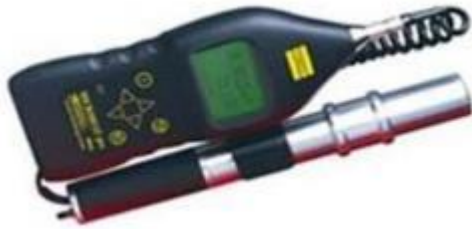
Photo 4-4: Instrument used – CASSELLA MicroDust to measure dust (TSP)
