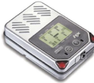
Photo 4-4: Instrument used – CASSELLA MicroDust to measure dust (TSP)
