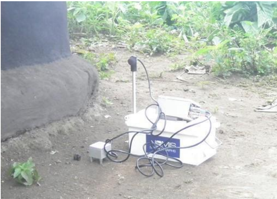
Photo 4-7: Field ground vibrations measurement using a Nomis Seismograph
