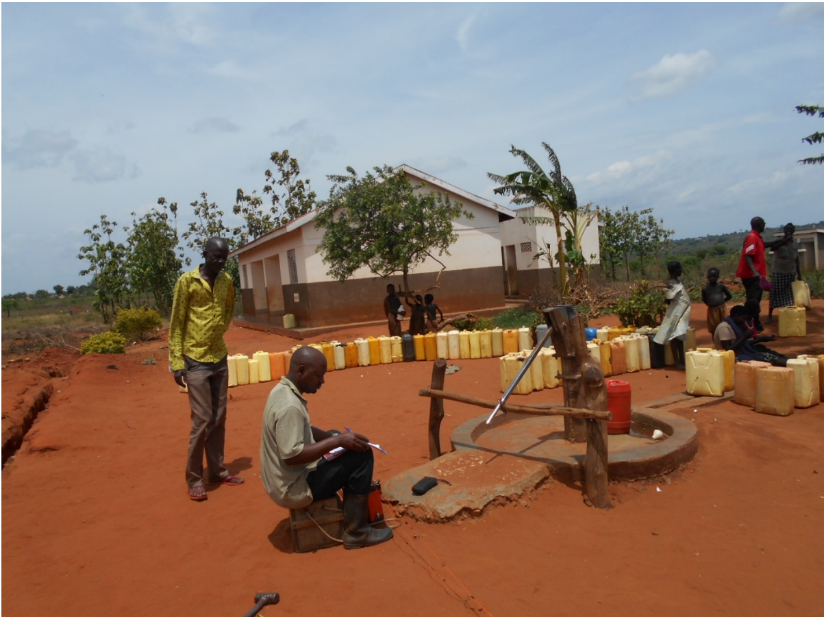
Calibration sounding at an existing borehole
