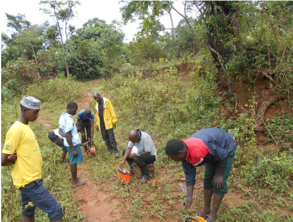
Set up of Resistivity surveys using Vertical Electrical Technique
