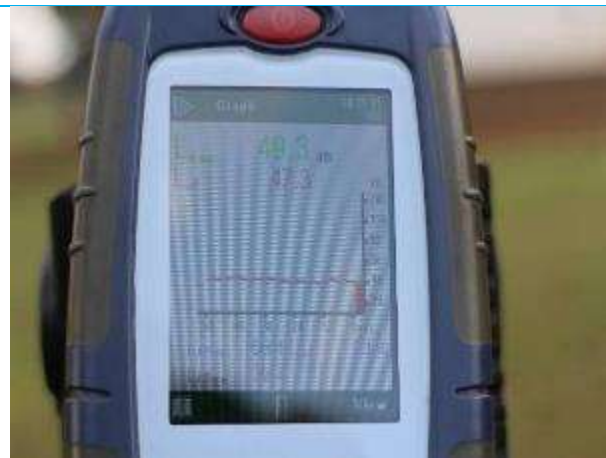
Display of results by Casella CEL-633B during measurement of ambient noise levels
