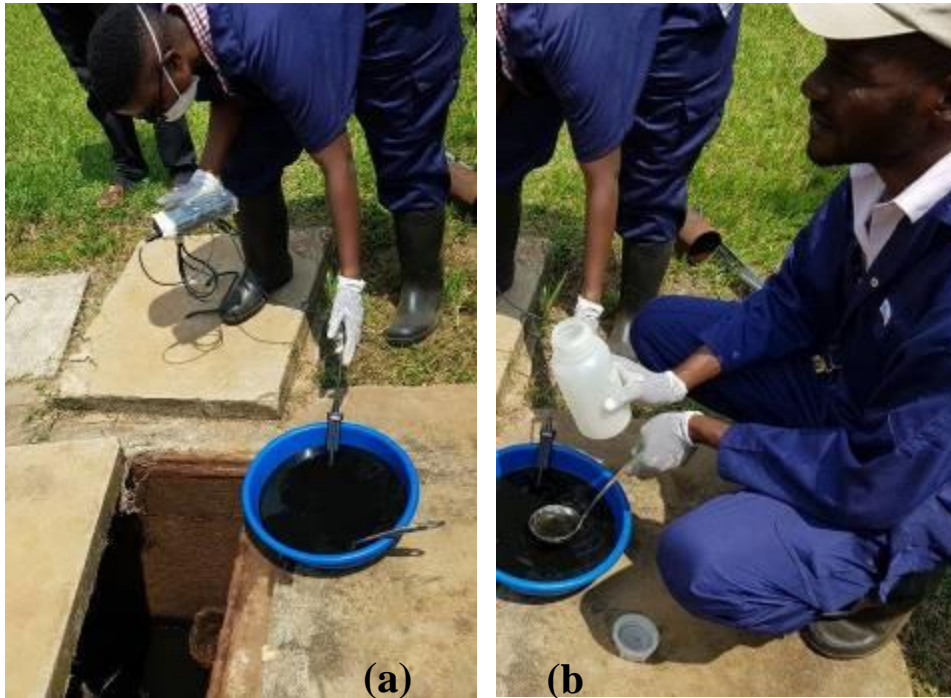
Figure 2-3: Faecal sludge sampling from (a) Pour flush toilet connected to a Cesspit, and (b) Lined pit latrine using a sampler
