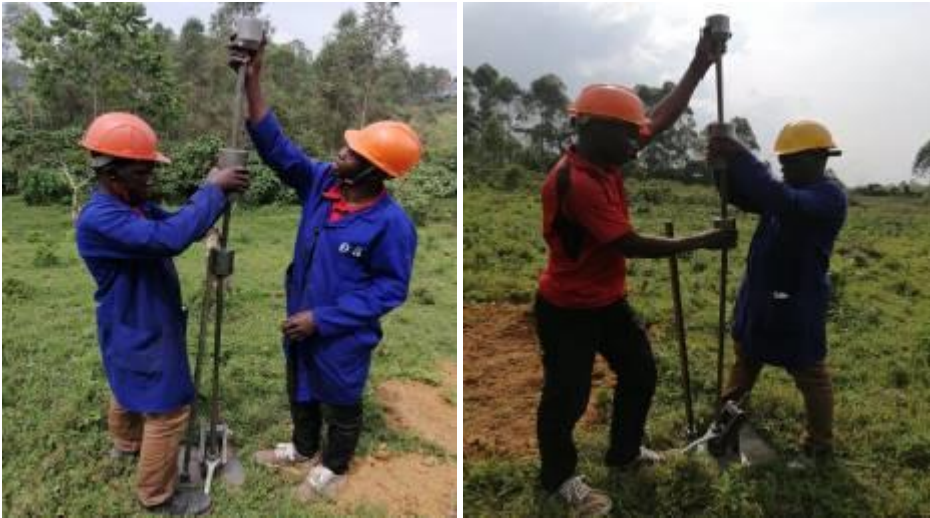
Figure 2-2: Conducting of the DPL test at site
