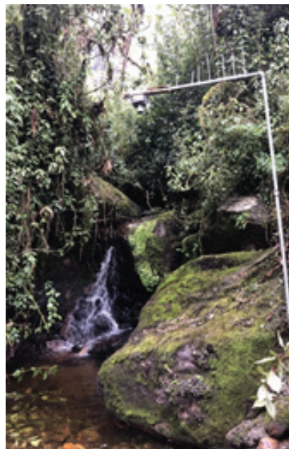
B: Water level sensor installed
