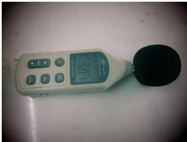
Plate 1: Noise level meter used for noise assessment. Taken on 10 th March 2023 by the Environmentalist
