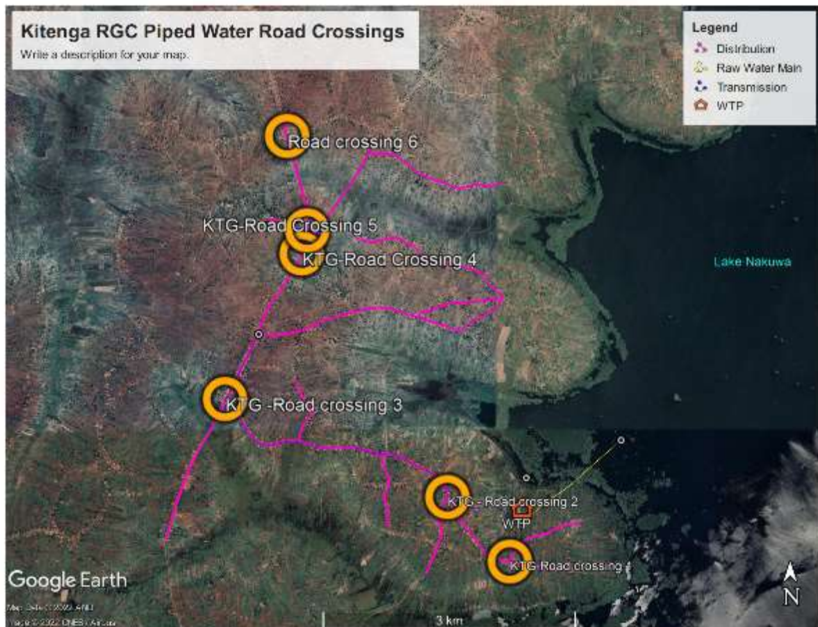
Figure 2-13: Major pipeline access road crossing
