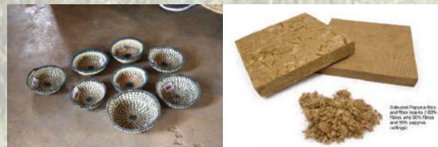
L-R Examples of traditional handcrafted papyrus baskets, Processed boards out of papyrus fibre prototyped by ZELFO Technology
