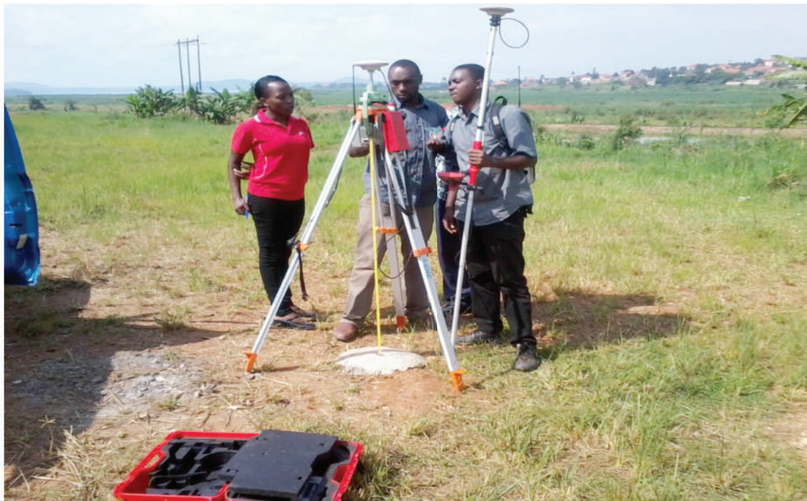
Plate 31: Wetland demarcation a) Wetland pillars used to demarcate wetlands, b) installed pillar at a wetland boundary, c) Setting controls before actual surveying and demarcation of wetlands
