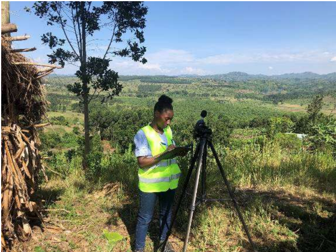
Photo 5-8 Ambient Air quality and Noise level measurements at Nakasero proposed reservoir point
