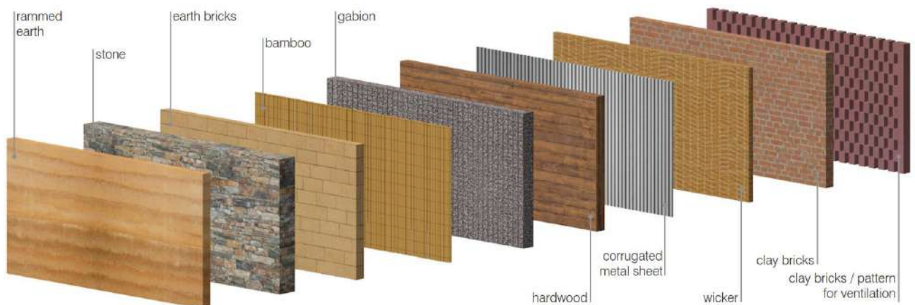
Figure 4.4: An overview of walls and space divisions that will be used depending on the location of the VIC
